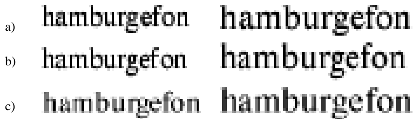
Fig. 6. (a) Component-based generation of grayscale characters, with improved contrast obtained thanks to phase control of stems and round parts and to thickness control of thin strokes; (b) Perceptually-tuned grayscale characters generated by applying hinting instructions to the grid-fitting process; (c) corresponding grayscale characters generated by filtering and resampling (traditional technique)
