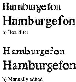
Figure 3. Characters generated by filtering and resampling compared with manually edited grayscale characters
