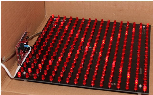
Figure 4 : 16 x 16 matrix LED display. Visible in the left, a Launchpad MSP430G is used to program the flash memory
