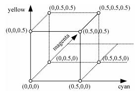
**Figure 1.** Illustration of the cellular Yule-Nielsen model where the illustrated cube represents one of the 8 subdomains produced by all combinations of 0%, 50% and 100% surface coverages of the three inks. At the vertices of the cube, subdomain primary reflectances  $R_{c.m.v}(\lambda)$  have been measured.
