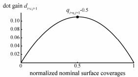
**Figure 2.** Cyan dot gain curve corresponding to the cyan ink spreading curve within the subdomain  $c,m,y \in [0,0.5]$ , for a cmy laser print (Brother 4000-HL) at a screen frequency of 120lpi and using an optimal n-value of 14.
