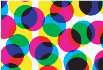
Figure 6. Colorants cyan, magenta and yellow generated by single inks printed on paper, colorants red, green and blue generated by the superposition of two inks and colorant black generated by the superposition of the three inks.
