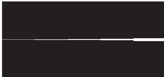
Figure 7.7: Test strip with a series of white micro-lines spaced out of a magenta solid patch. The line thickness ranges between 100 \mu m and 1 mm .
