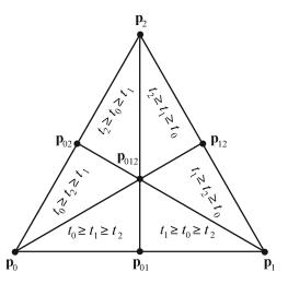
Figure 12. Characterization of each subdivided simplex using the inequalities of the barycentric coordinates.
