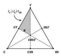
Figure 5. A single point **x** with barycentric coordinates  $t_r \ge t_c \ge t_m$  has to be interpolated within the corresponding highlighted subsimplex defined by cellular primaries **r**, **cr** and **cmr**.
