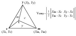
Figure 6. The area-coverage of the halftone represented with the vector  $\mathbf{t}$  (*c*, *m*, *y*) is equal to the relative area of the three opposite-side sub-triangles.
