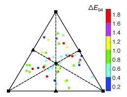
Figure 8. The  $\Delta E_{94}$  color prediction error for a number of 3-ink halftones predicted with the cellular simplex YNSN. The test halftones are shown with filled circles color-coded according to the prediction accuracy error. The location of the measured calibration samples is also shown with black shapes: The fulltone inks are shown with squares, the two-ink cellular primaries are shown with triangles and the 3-ink cellular
