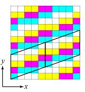
Figure 7. Discrete-line juxtaposed halftoning: a simple example of a screen comprising four colorants with different areacoverages: cyan 25%, magenta 20%, yellow 25% and white 30%. Two instances of the parallelogram screen-element are shown with a solid line. Here the vertical period T is 4 and the line slope is 2/5.
