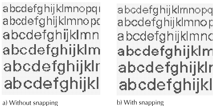
Figure 23. Rasterization of unregularized Haas-Unica
