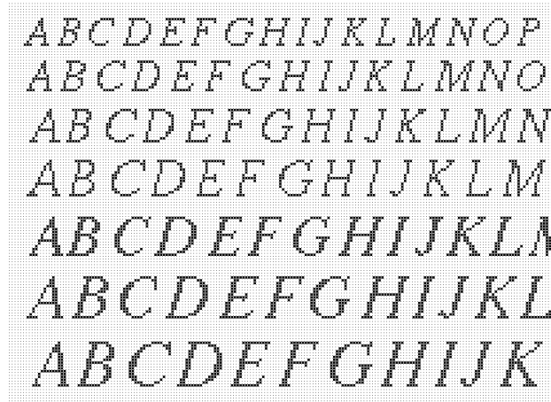
Figure 27. Rasterization of automatically hinted italic outline characters
