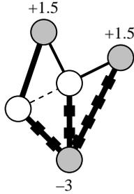
**Fig. 2.** Remove the bottleneck links from the network, adjusting the flow-out coefficients at the adjacent nodes, maximize the flow in the new sub-problem, fix the new flow-out coefficients at the nodes and find the new bottlenecks (layer 2,  $F^2 = 1.5$ )
