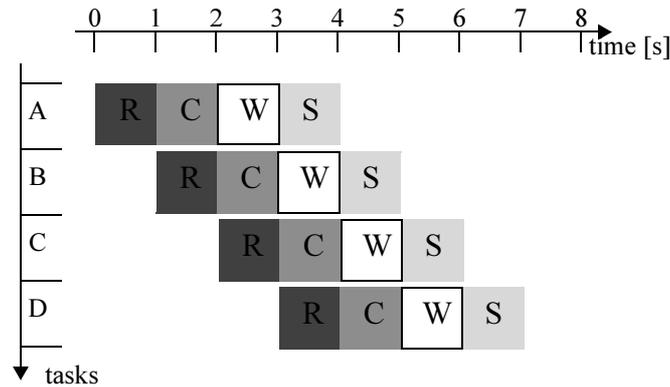
Fig. 2.5 Executing the encryption program in pipeline (1 MB blocks)
