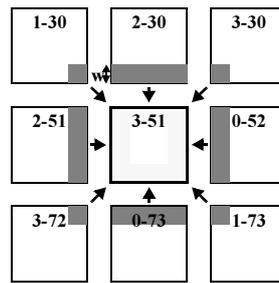
Fig. 7.10 Borders exchanged during a neighborhood dependent operation
