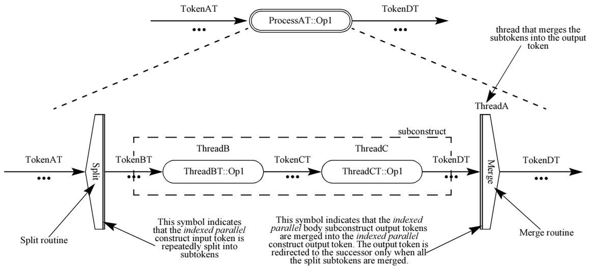
Fig. 3.23 Graphical CAP specification of the *indexed parallel* construct
