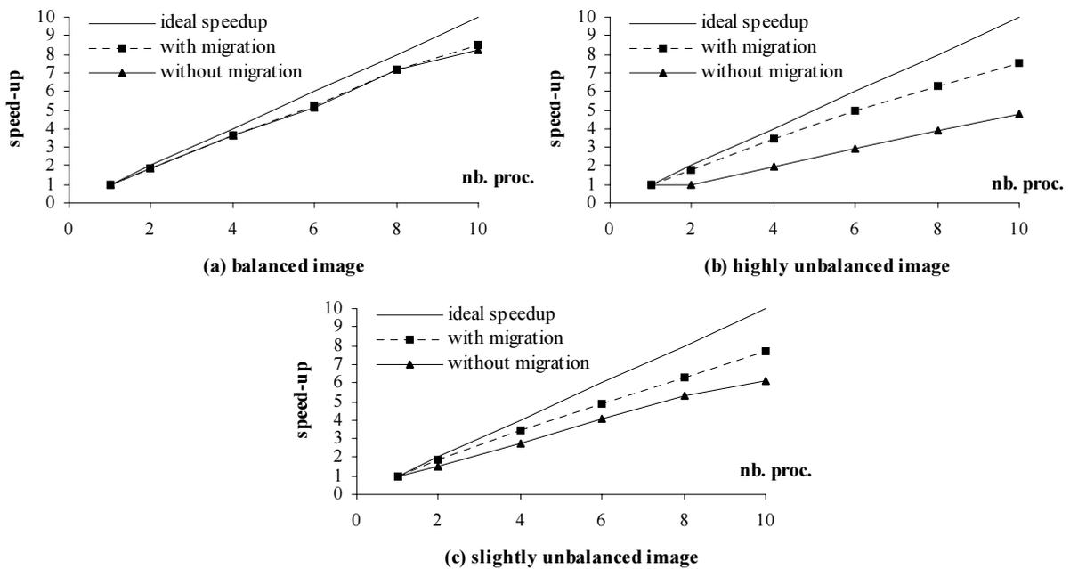
Fig. 8.7 Speedup for (a) the balanced input image, (b) the highly unbalanced input image and (c) the slightly unbalanced image
