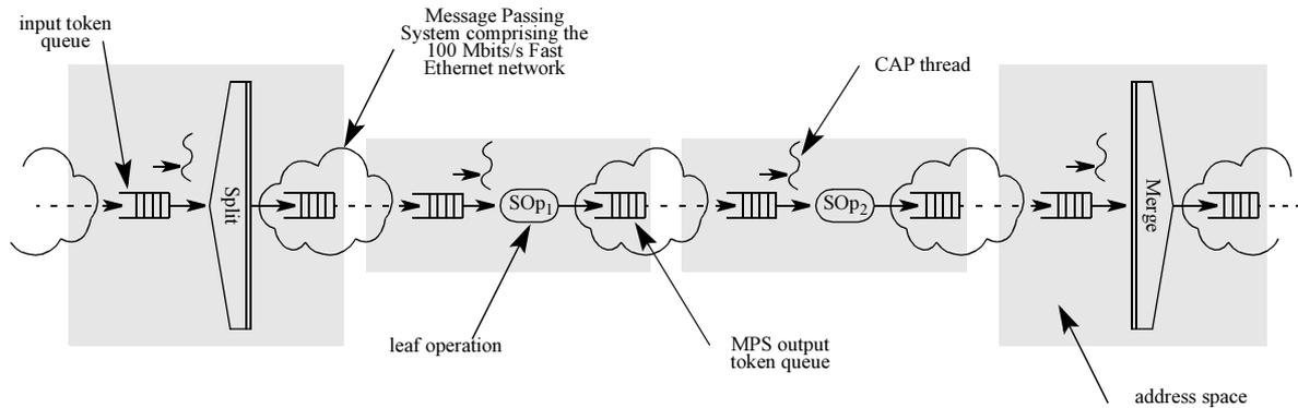
**Fig. 4.1** Example of a 4-stage pipeline composed of a split routine, two intermediate leaf operations and a merge routine. Note the input token queues in front of each CAP threads and the MPS output token queues at the border of each address spaces.
