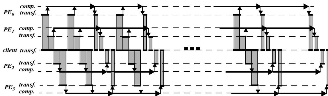
Fig. 6.1 Dynamic matrix multiplication: timing diagram
