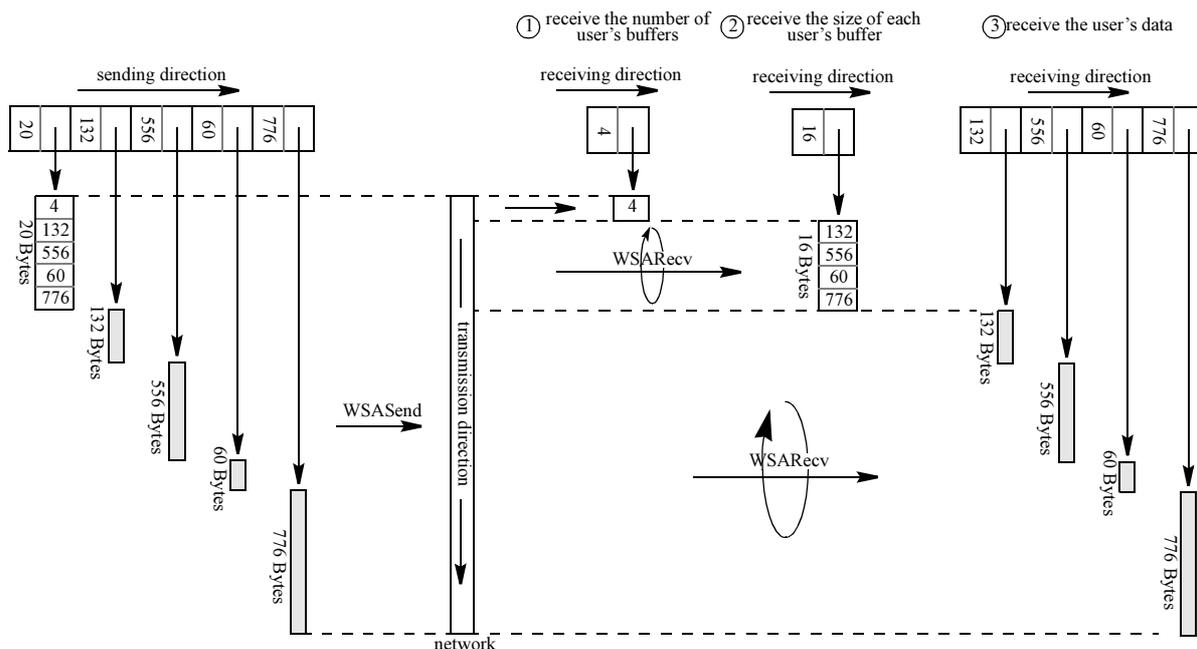
**Fig. 5.2** The three steps mechanism that enables a scattered packet to be transmitted from one address space to another using a stream socket (TCP/IP protocol) and the overlapped gather/scatter *WSASend* and *WSAREcv* routines
