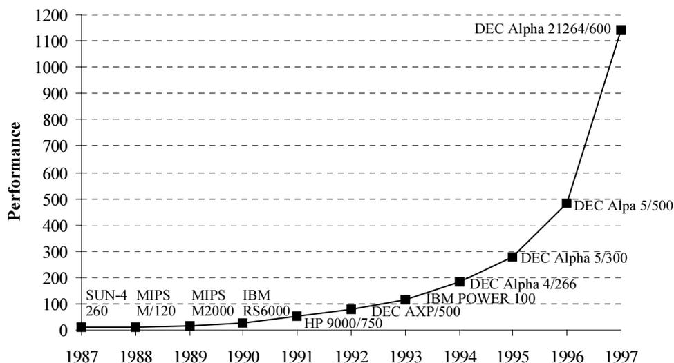
**Fig. 1.1** Performance increase of workstations, 1987-1997. Here performance is given as approximately the number of times faster than the VAX-11/780, which was a commonly used yardstick. The rate of performance improvement is about 1.54 per year, or doubling every 1.6 years. These performance numbers are from the integer SPEC92 benchmarks (SPECbase\_int92) except the two later machines based on the SPECin95base and multiplied by a factor to estimate SPECbase92 performance.
