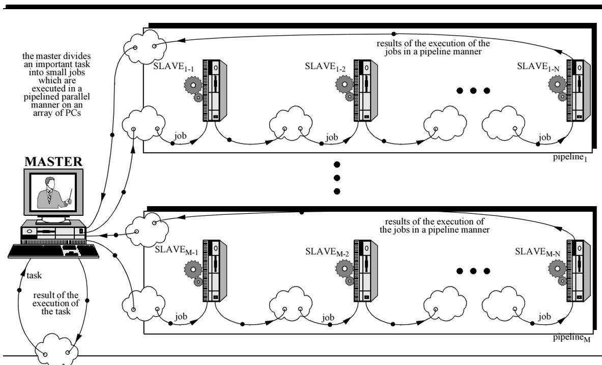
**Fig. 4.7** Execution in a pipelined parallel manner on a multi-PC environment
