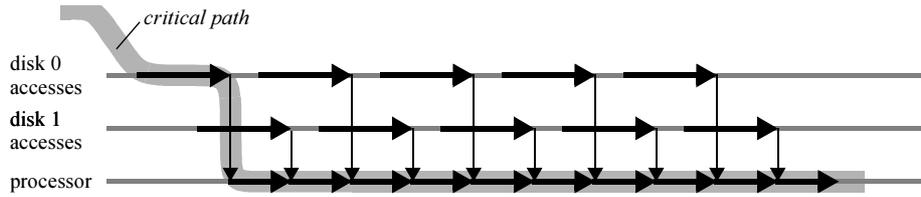
Fig. 7.6 Execution schedule with a single PC and two disks (processor bottleneck)
