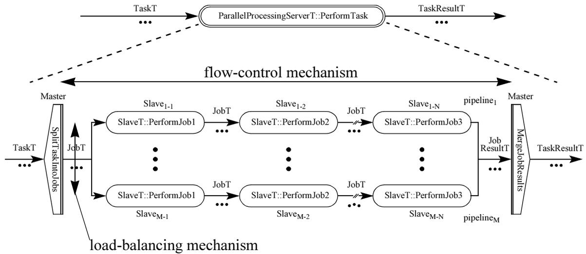
**Fig. 4.8** Graphical representation of a pipelined parallel execution. The horizontal arrow represents the flow-control mechanism and the vertical arrow represents the load-balancing mechanism
