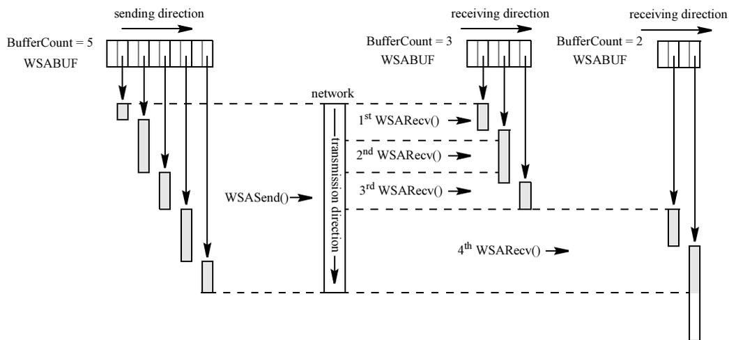
**Fig. 5.1** The TCP protocol has no notion of packets. There is no correspondence between the *WSASend* and *WSARecv* calls.
