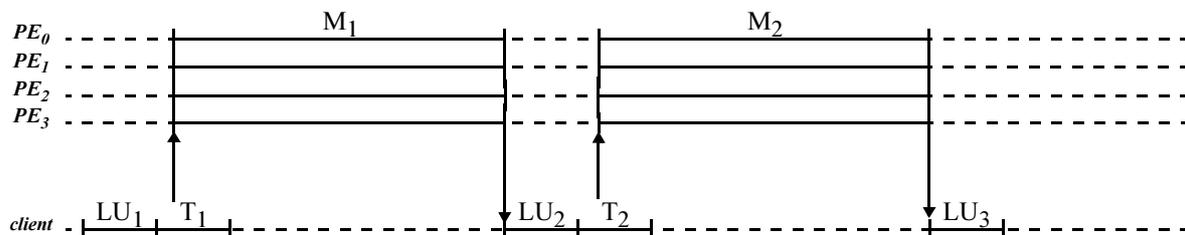
Fig. 6.4 LU factorization with pipelined matrix multiplication
