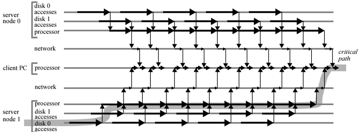
Fig. 7.7 Execution schedule (multiple single-processor PCs with two disks, slave processor bottleneck)
