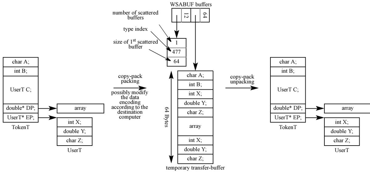
Fig. 5.3 The copy-pack serialization uses a temporary transfer buffer to copy the structure's data so that the data encoding can be modified
