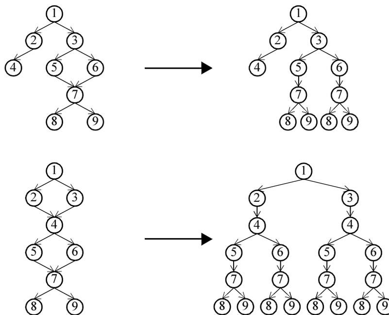
Fig. 10.2 Unfolding graphs into trees
