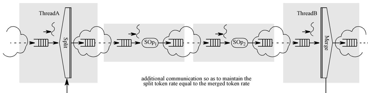
**Fig. 4.2** High-level flow-control mechanism requiring additional communication between the thread that runs the merge routine (the ThreadB thread) and the thread that runs the split routine (the ThreadA thread) so as to maintain the split token rate equal to the merged token rate
