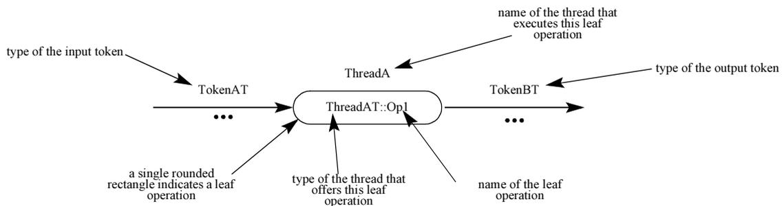
Fig. 3.12 A leaf operation with its input and output token. Single rounded rectangles depict leaf operations
