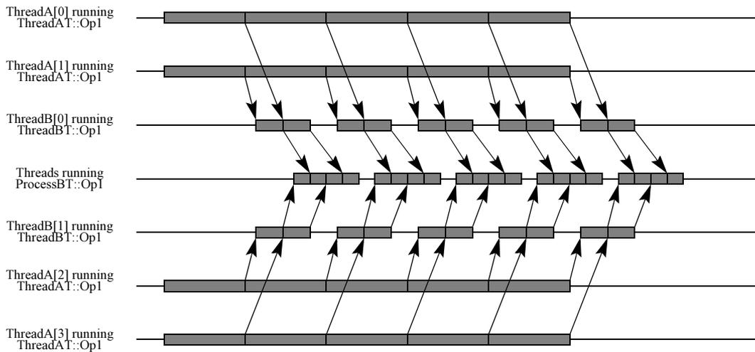
Fig. 3.21 Timing diagram of a pipelined parallel execution
