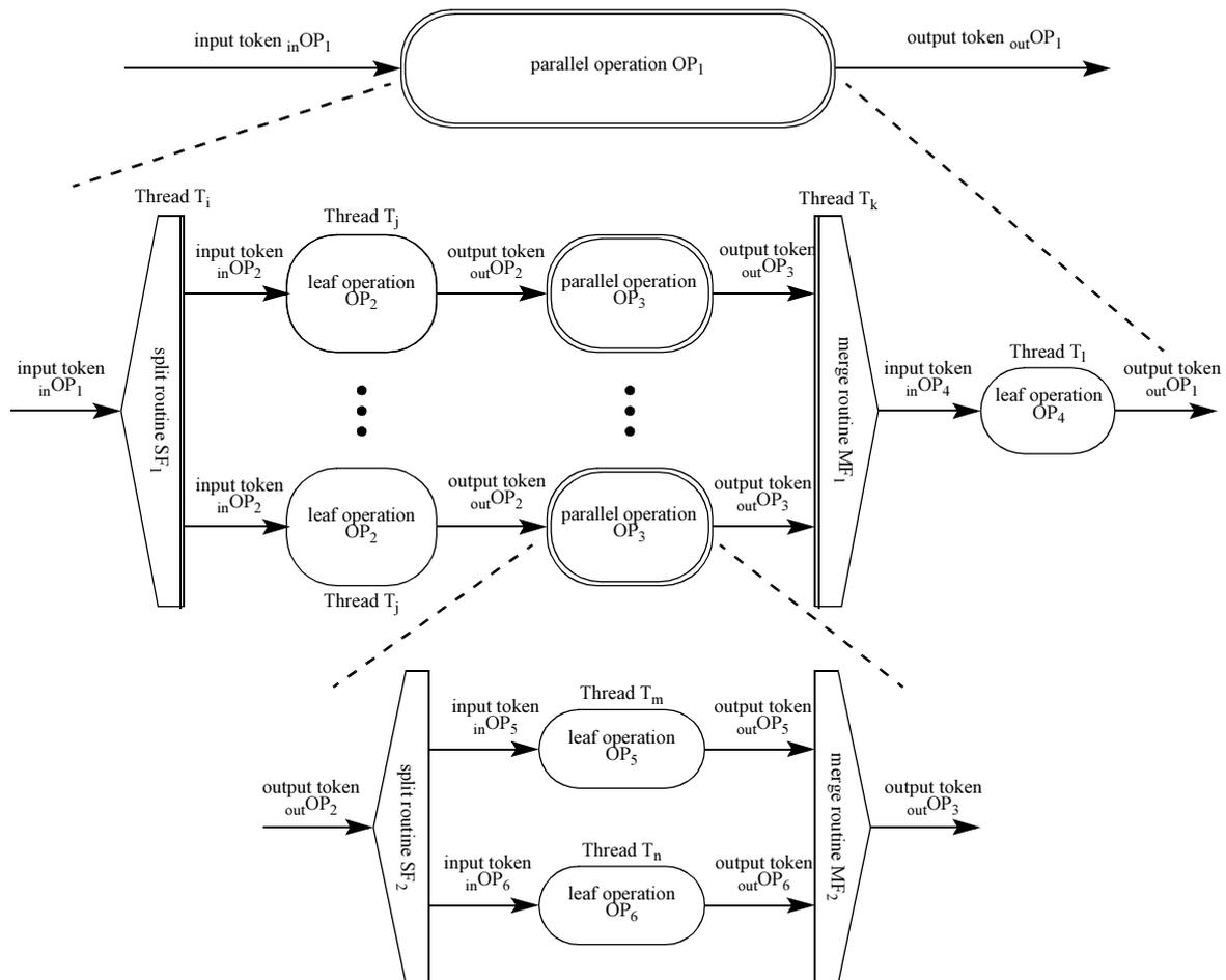
**Fig. 3.3** Graphical CAP specification: parallel operations are displayed as parallel horizontal branches, pipelined operations are operations located in the same horizontal branch
