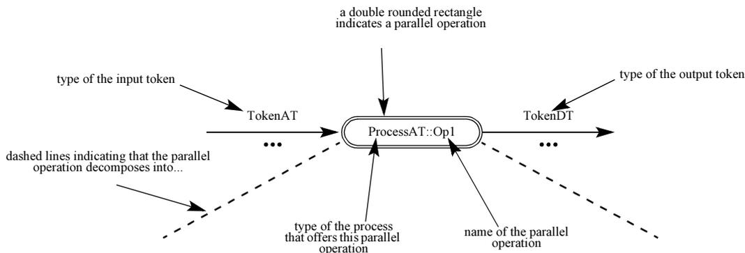
Fig. 3.14 A parallel operation with its input and output token. Note double rounded rectangle depict parallel operations.
