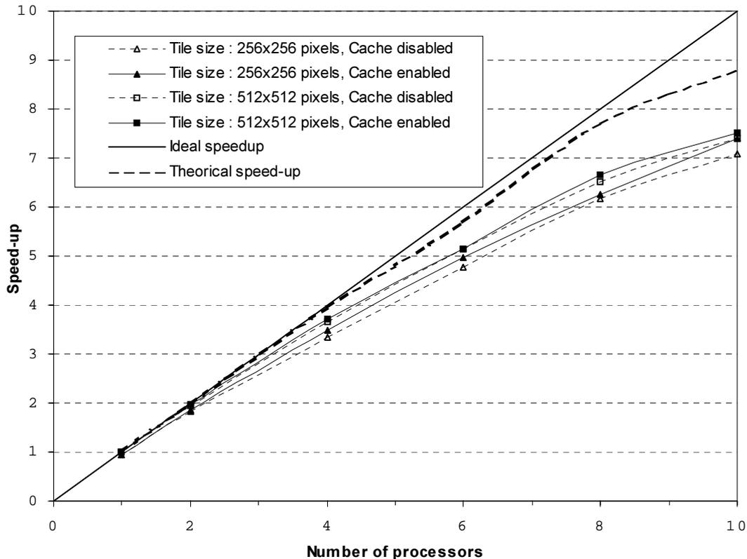
Fig. 7.14 Speedup as function of the number of processors
