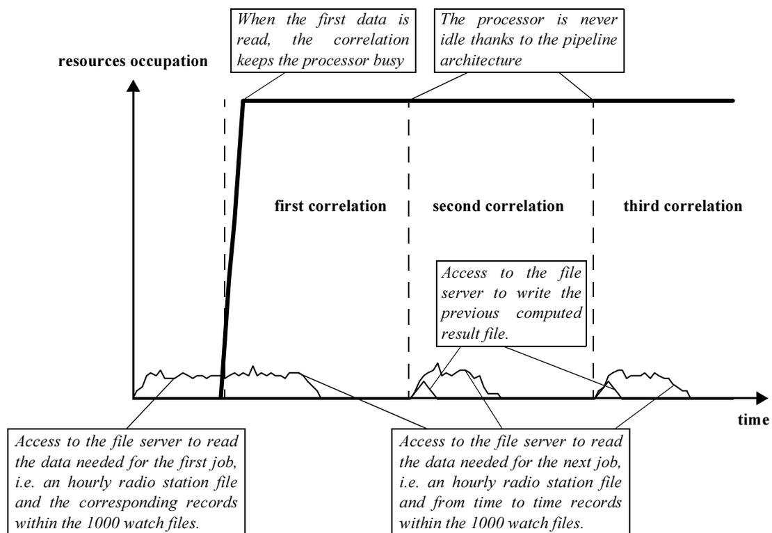
**Fig. 9.4** Slave activity during the correlation process: the thick line represents the processor occupation on the slave, and the thin lines represent the file server accesses
