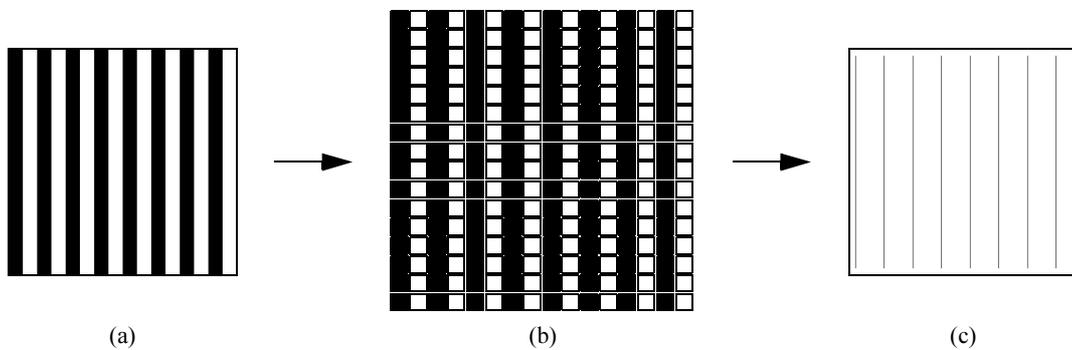
**Fig. 8.9** Example (a) of a highly unbalanced input image, (b) after segmentation into cells and (c) after skeletonization
