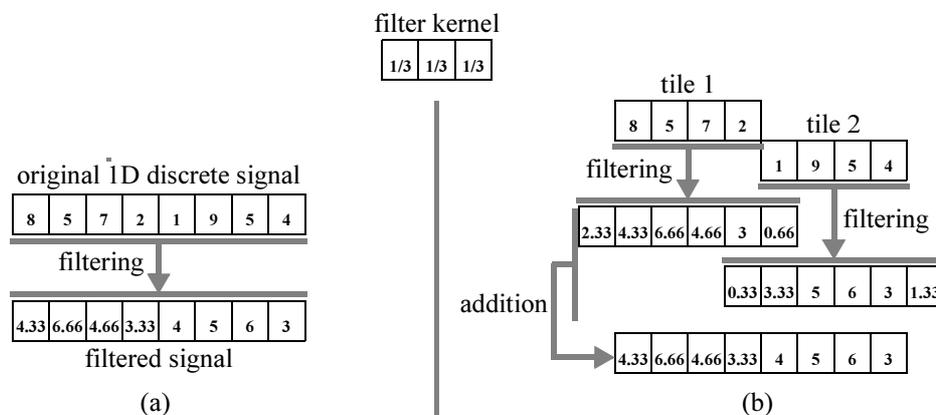
Fig. 7.5 Applying a linear filtering operation to a 1-D discrete signal.
