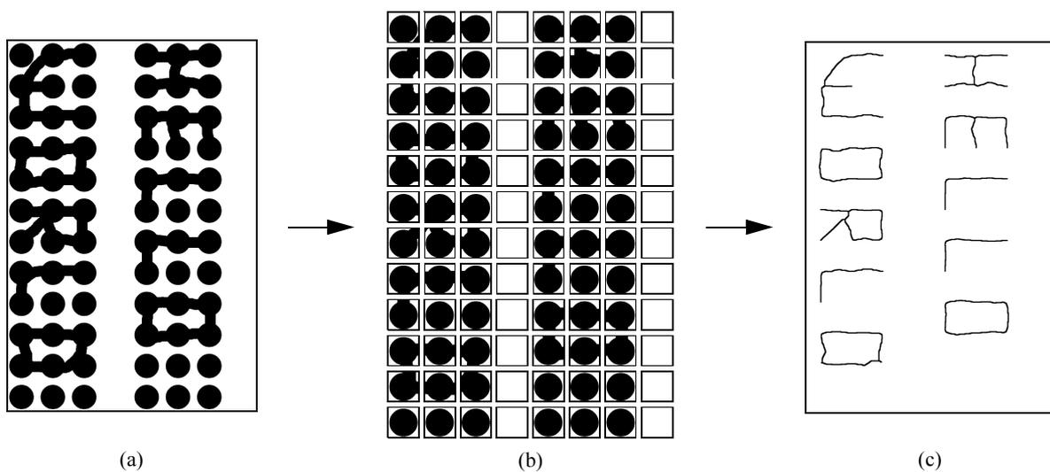
**Fig. 8.10** Example (a) of a slightly unbalanced input image, (b) after segmentation into cells and (c) after skeletonization
