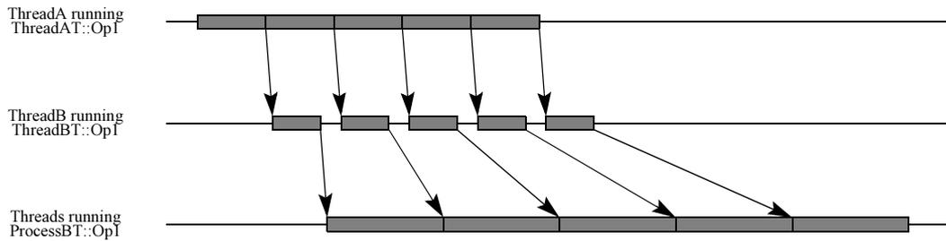
Fig. 3.18 Timing diagram of the execution of the 3 operations in a pipelined manner
