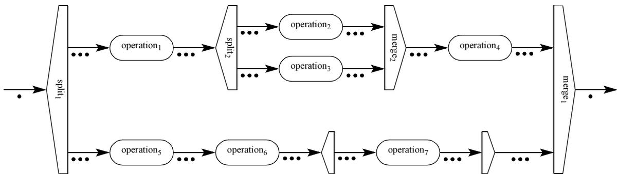
**Fig. 3.1** An example of a CAP macro-dataflow depicted by a symmetric directed acyclic graph. Arcs model data dependencies between operations. Tokens carry data along these arcs. Split routines split input tokens into several sub-tokens sent in a pipelined parallel manner. Merge routines merge input tokens into one output token thus acting as synchronization points
