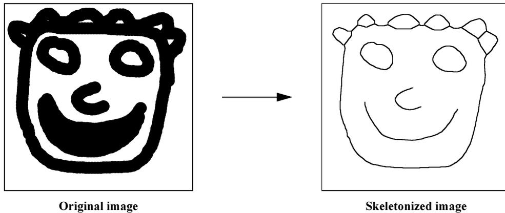
**Fig. 8.1** Skeletonization algorithm example
