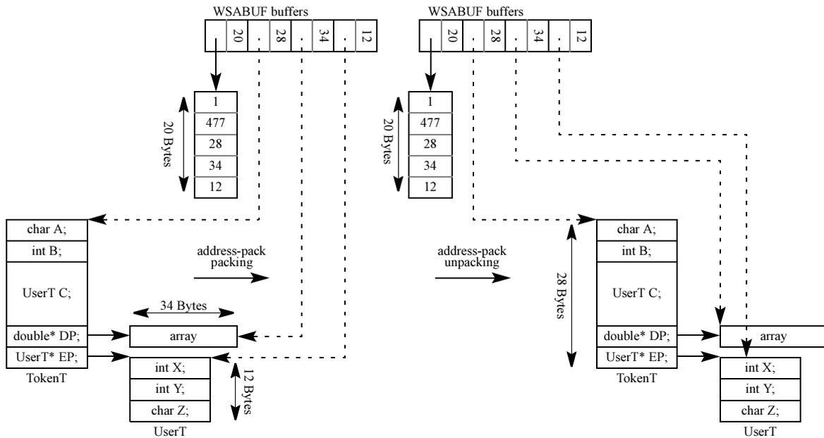
Fig. 5.4 The address-pack serialization uses a list of scattered buffers for sending and receiving the structure's data with no memory-to-memory copy
