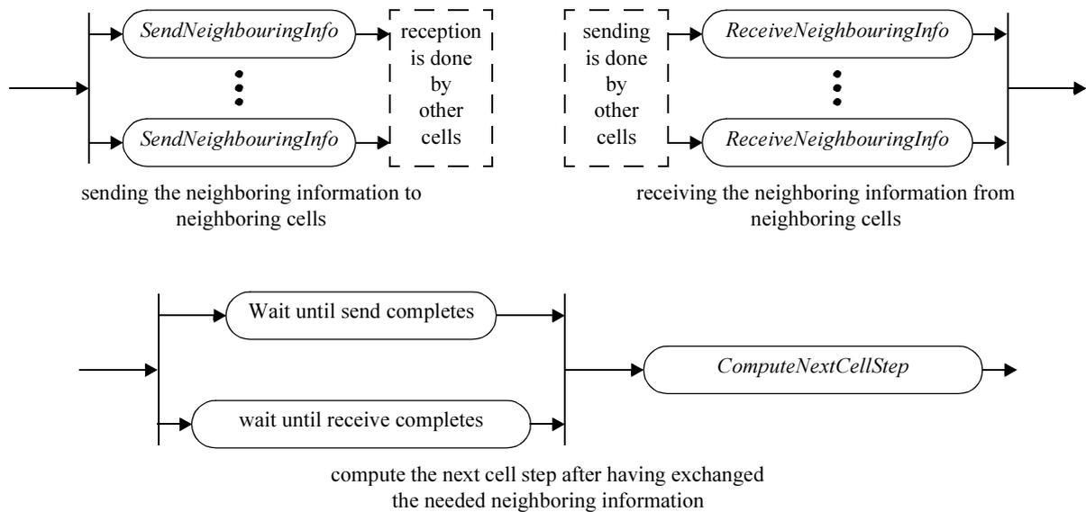
Fig. 8.4 Parallel skeletonization algorithm schedule for one cell
