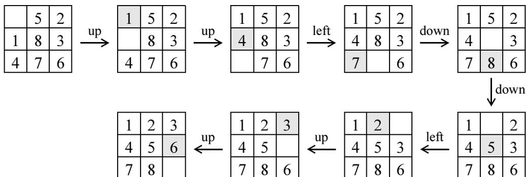
**Fig. 10.1** An Eight-puzzle problem instance: sequence of moves leading from the initial to the final configuration
