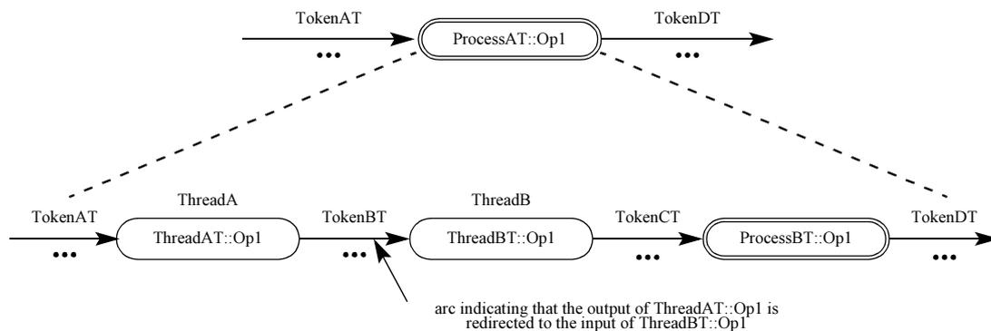
Fig. 3.16 Graphical CAP specification of the *pipeline* construct
