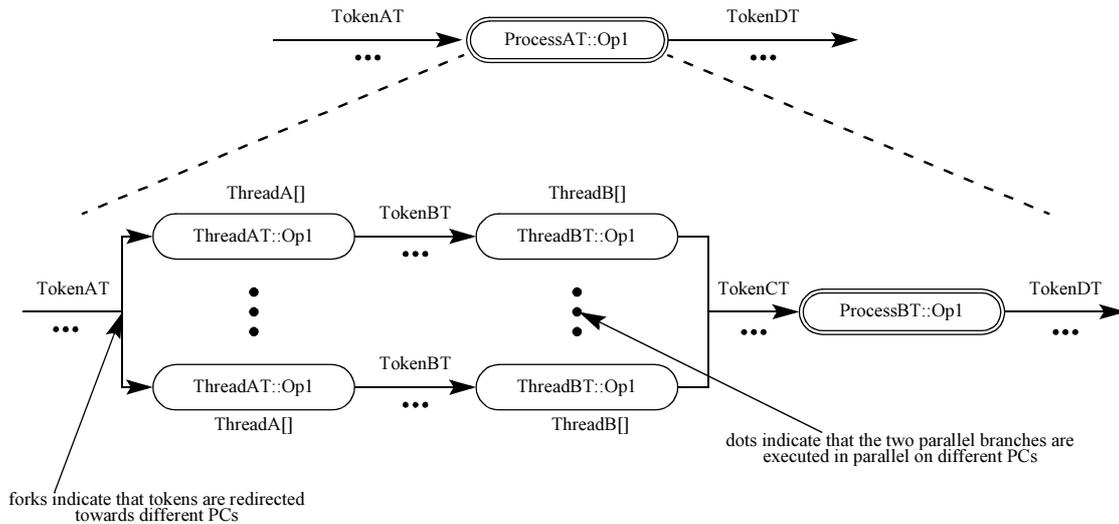
Fig. 3.22 Graphical representation of a pipelined parallel execution
