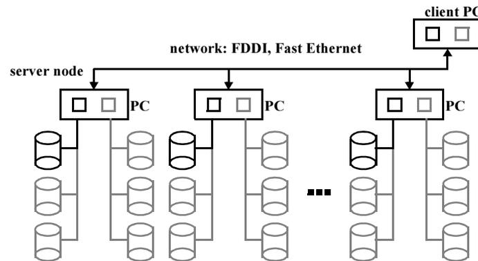
Fig. 7.1 Commodity component based parallel architecture composed of one client node and several server nodes
