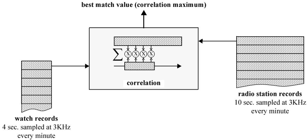
Fig. 9.2 Global scheme describing the matching process
