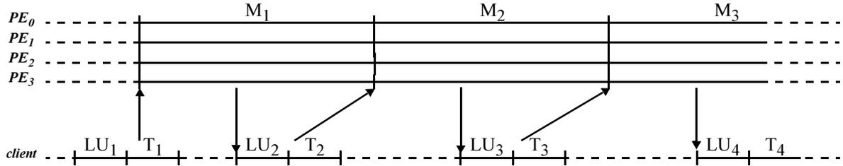
Fig. 6.5 LU factorization with full pipelining
