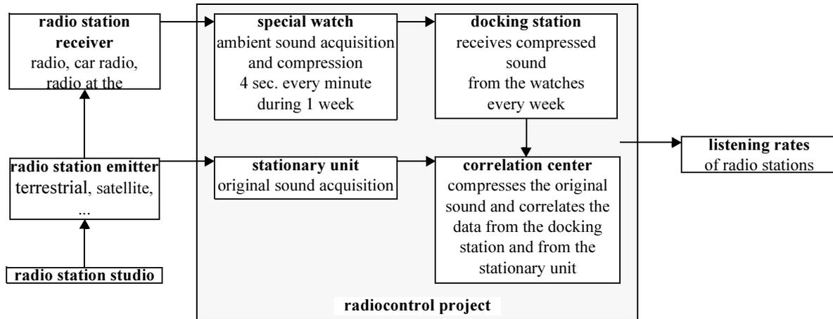
Fig. 9.1 Complete data flow from the radio emitter to the correlation center
