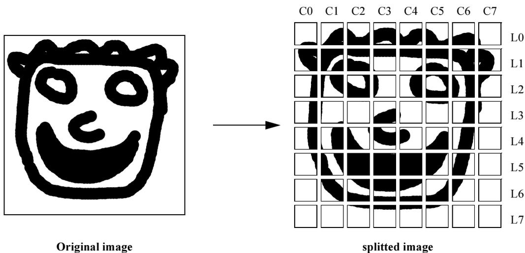
Fig. 8.3 Division of the input image into cells
