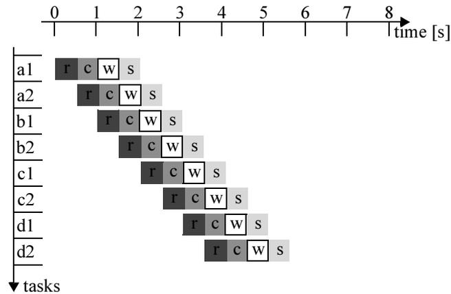
Fig. 2.6 Executing the encryption program in pipeline (0.5 MB blocks)
