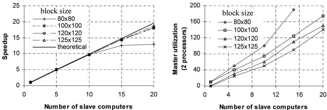
Fig. 6.6 Matrix multiplication speedup and client computer utilization (1000x1000 matrices)
