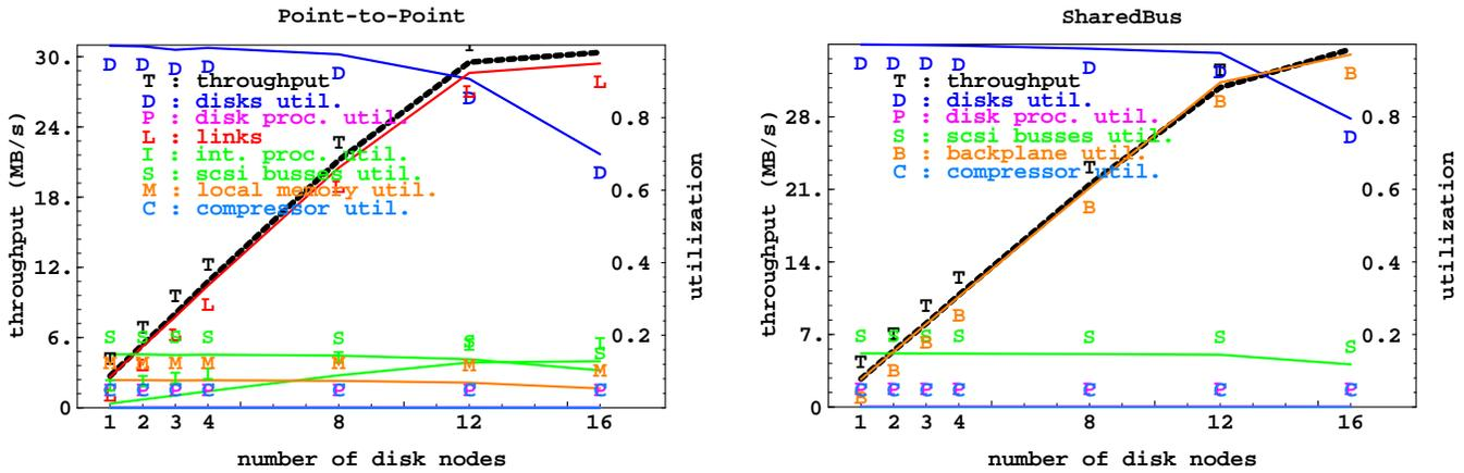
Figure 4 : Reading streams : throughput and utilization
