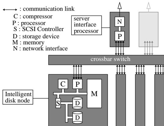
Figure 2 : Point to point architecture
