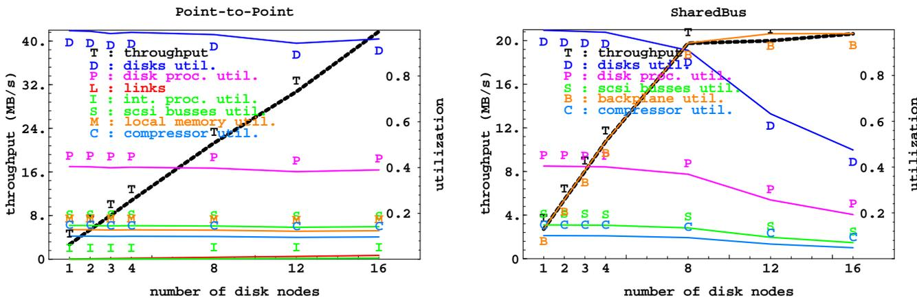
Figure 6 : Resampling uncompressed streams: throughput and utilization
